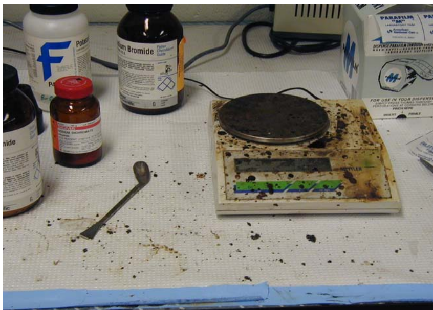
Apparent spill of ethidium bromide onto lab bench and balance
